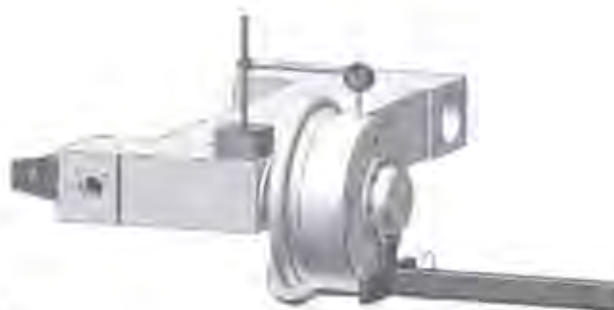
FIG 1. ATTACH MAG-BASE SECURELY TO FRAME.
