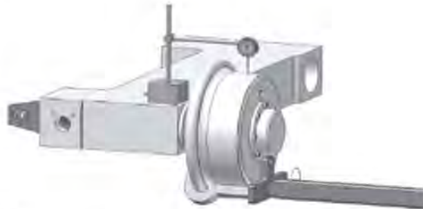
FIG 1. ATTACH MAG-BASE SECURELY TO FRAME.
