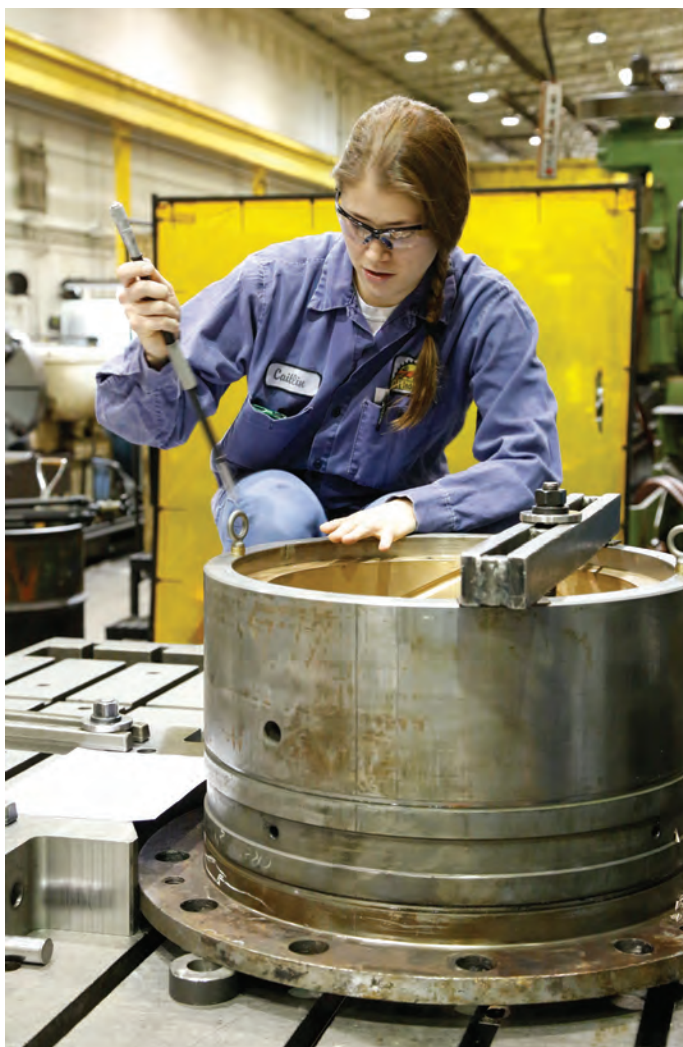
Above: A team of L&H engineers, welders and project coordinators with a 48-foot boom sent to a customer in Mexico. Left: L&H machinist Caitlin Fox measures a bushing prior to machining.
